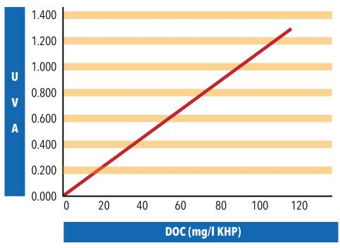
UV-254 measurements are a practical indicator of dissolved organic compounds in water. Traditional methods such as TOC, COD, and BOD all capture more organics and other potential contaminants but have the drawback of being expensive and maintenance intensive. In fact, most are done only in the laboratory due to the complexity of on-line systems.
