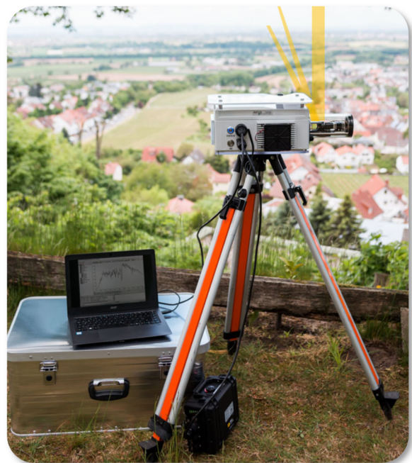
SkySpec Mini in the field with tripod and LiPo battery pack (available accessories)
