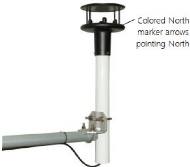
FIGURE 7-1. WindSonic1 mounted on a crossarm
