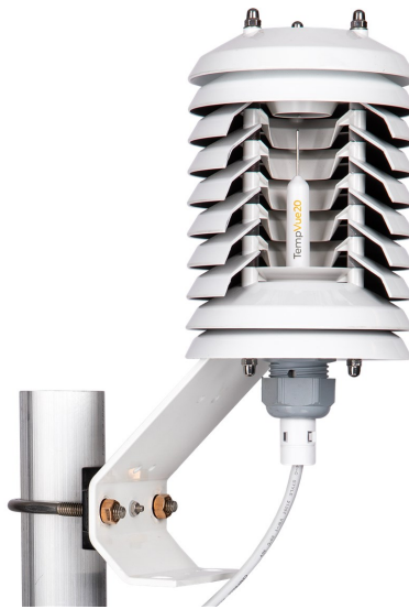
Figure 7-2. Cut away view shows TempVue 20 SDI-12 insertion in a RAD shield
