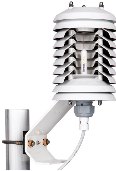
Figure 7-2. Cut away view shows TempVue 10 insertion in a RAD shield
