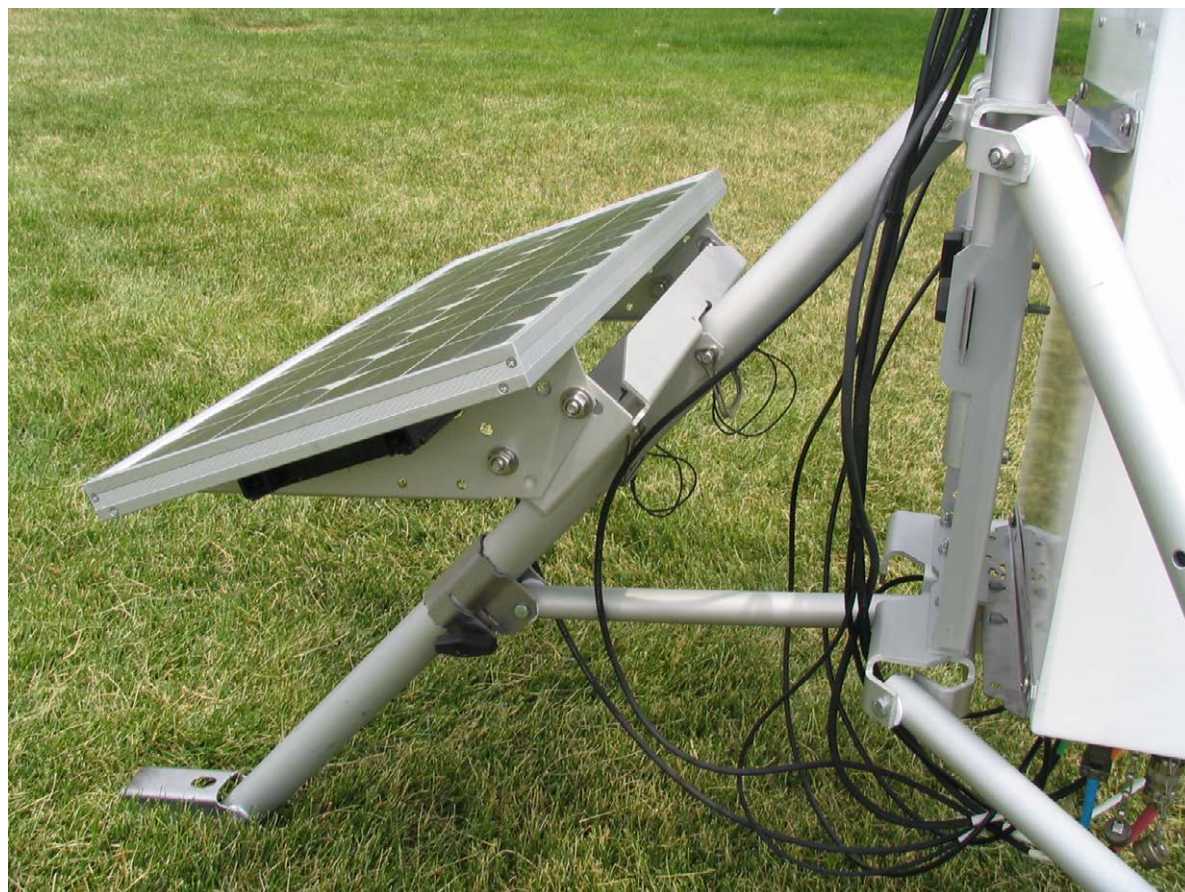
Solar panel should face the equator.
