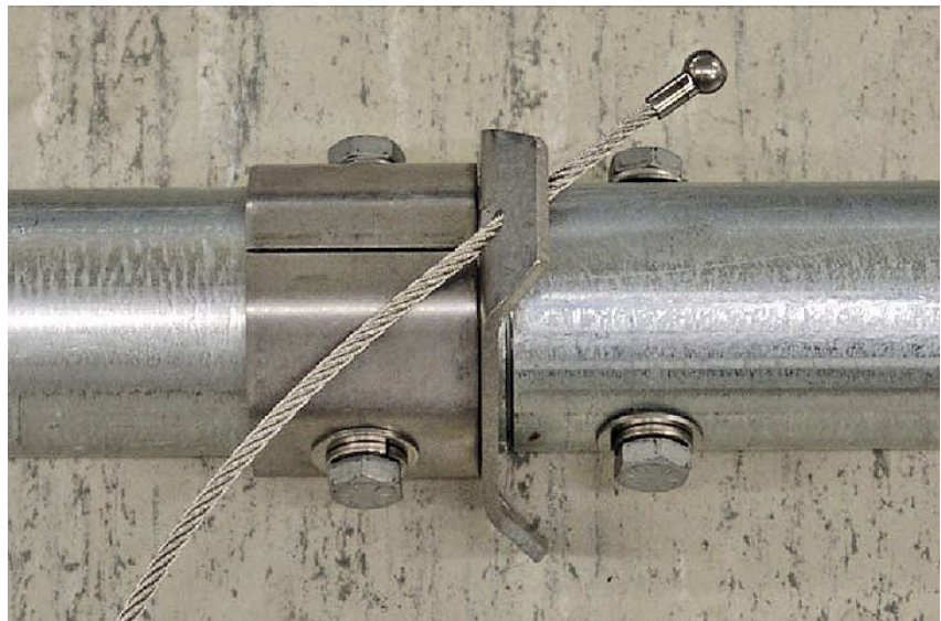
FIGURE 3-16. Mast Section 5 and guy ring/collar assembly
