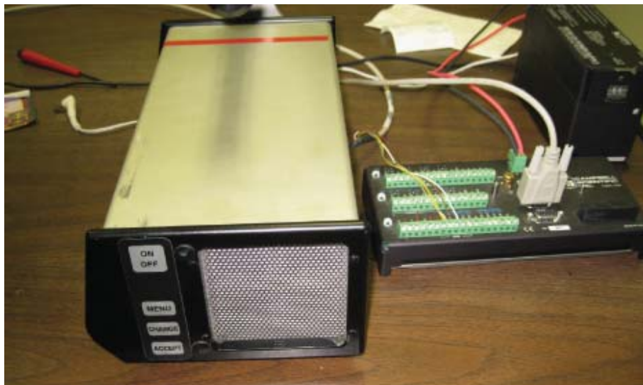
Figure 2. Above shows the AlphaGUARD connected to a CR1000 datalogger.
