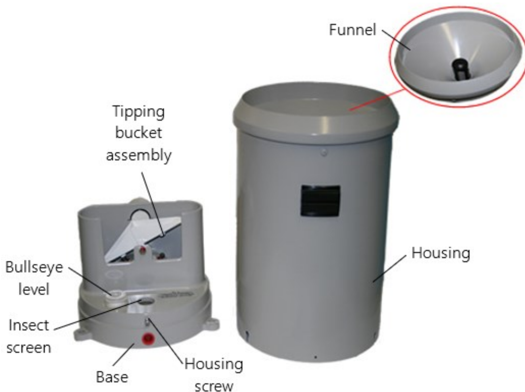
Figure 9-1. Main components of the CS700
