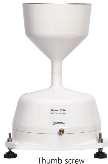
Figure 7-3. Thumb screw on RainVUE 20
