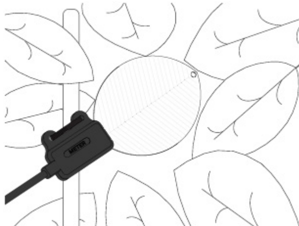
FIGURE 7-2. Top view of a typical LWS installation
