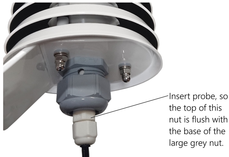
Figure 7-1. HygroVUE 5 detail of insertion in a RAD06 shield
