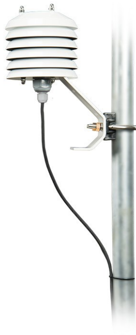
Figure 7-2. HygroVUE 5 installed in a RAD06 radiation shield on a pole
