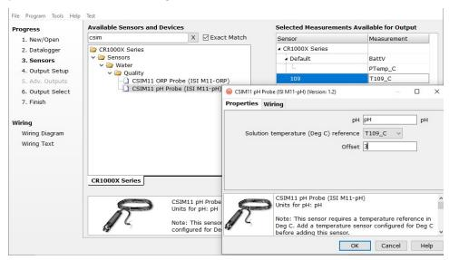
6. Click the **Wiring** tab to see how the sensor is to be wired to the data logger. Click **OK** after wiring the sensor.
