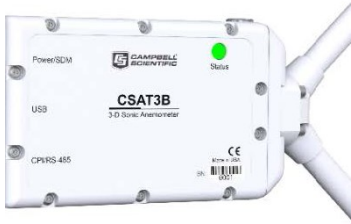
Figure 6-12. Lit status light on CSAT3B block
