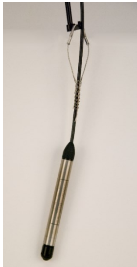
Figure 7-1. Transducer suspended with split mesh cable grip
