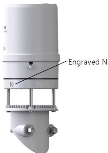
Figure 7-3. Engraved N on the ClimaVUE 50
