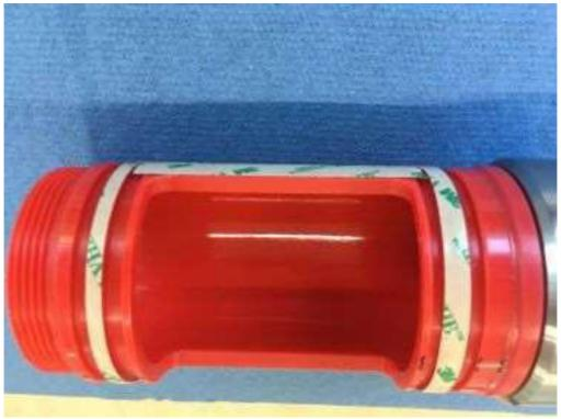
Take of the protection paper of the self-adhesive tape but without removing it completely.
