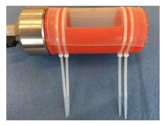
Finally, the overlapping mesh has to be cut-off carefully. In addition, the .flaps of the tie raps have to be cut-off, Please mind that the cut should be as close as possible to the lock of the tie raps in order to avoid sharp edges which might damage the net during use.
