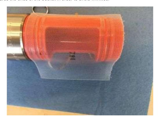
Finally remove the rest of the protection paper and press the rest of the mesh to the self-adhesive tape. Repeat applying pressure along the self-adhesive tape once again.
