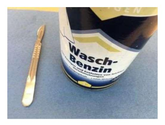
As a first step, the old mesh has to be removed from the net bucket, Please cut off the old tie raps and remove the mesh from the self-adhesive tape. Afterwards please also remove the old self-adhesive tape from the bucket and clean the bucket thoroughly with the cleaning solvent.
