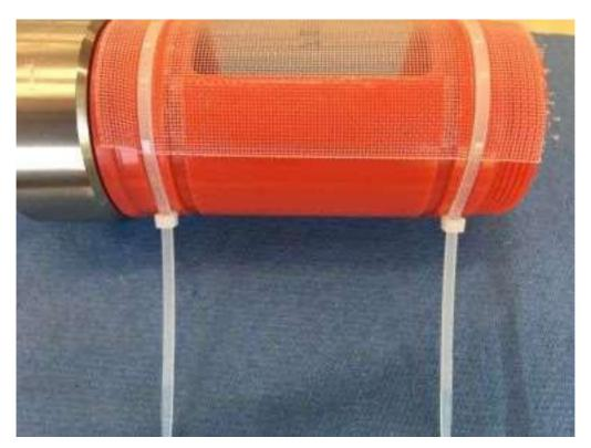
Now install the tie raps to the inner notches and fix them firmly.
