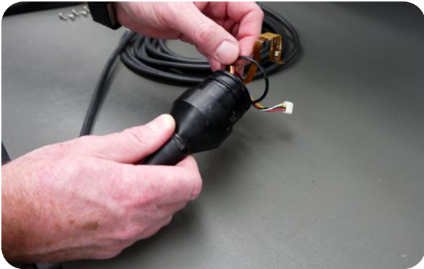
Cable and probe assembly seal replacement
