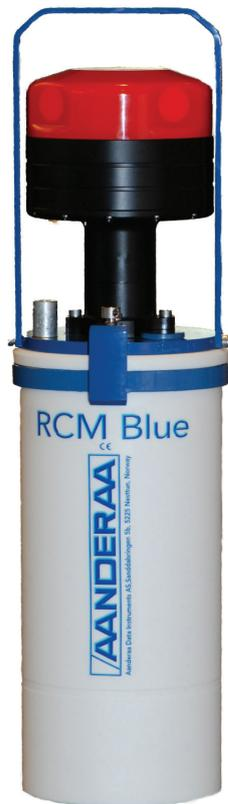
The RCM Blue is a self-recording Current Meter which also measures water temperature.
