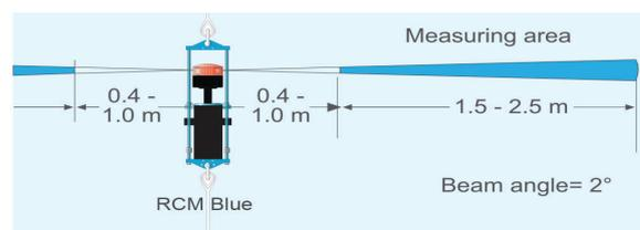
The solid state sensor is well suited for monitoring low current speeds due to no moving parts. Because the sensor starts measuring in an area 0.4 to 1.0 meter from the instrument, the effect of marine fouling and local turbulence is minimized.
