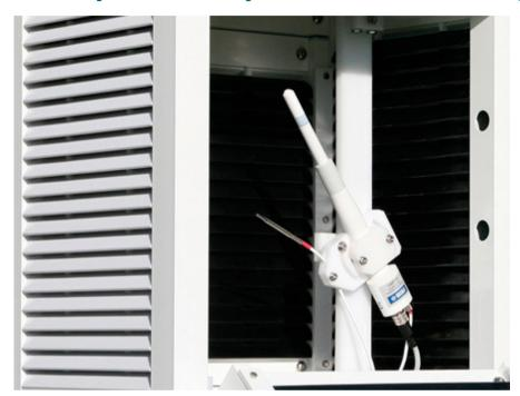
In high humidity climates where moisture is near saturation and in environments with changing temperatures, capturing accurate data is especially challenging. These are the types of conditions for which Vaisala's HUMICAP Humidity and Temperature Probe HMP155 were specifically designed.
