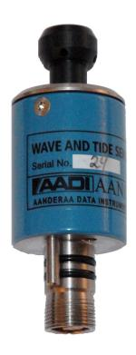
5218/5218R is based on a silicon piezoresistive pressure sensor. The pressure measurements are sampled and temperature compensated by an advanced Digital Signal Processor.
