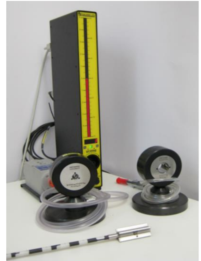
Hiden's Quadrupole air gauging tool
